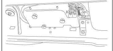
Mount Front and Rear Bracket using hardware removed from step 5.
