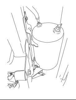
Mount Front and Rear Bracket. Rear bracket will Re-Use hardware removed in step 1. Front bracket will use provided flat head screw(6).
