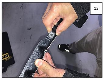
Attach 2 supplied Short "U" Clips to the supplied Front Inner Bracket as shown.
