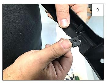
Attach 2 supplied Short "U" Clips to the supplied Top Inner Bracket as shown.
