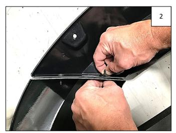
Install extension pieces to main front flares using 2 supplied #8 Speed Clips and #8 Truss Head Screws per side.
