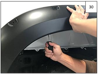
Start 3 supplied Truss-Head Screws through upper holes in flare and into clips installed in Step 28. Apply pressure to flare towards vehicle body at each fastening point and tighten all fasteners.
