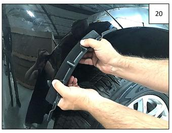
Use thumbs to fully press tape against vehicle, working along part.
