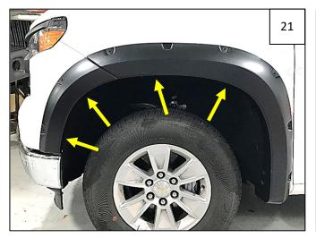
Align flare on vehicle and start 4 supplied Truss-Head Screws through holes in flare and into fender as shown.
