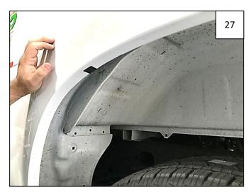
Peel liner from a supplied Foam Tab and center tab over each mark made in Step 25; fold each tab over lip of wheel well.
