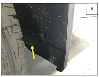
Using a 10mm socket, remove 1 factory bolt from mud flap indicated by arrow. Remove mud flap by pulling firmly away from vehicle body (a hidden clip will disengage).
