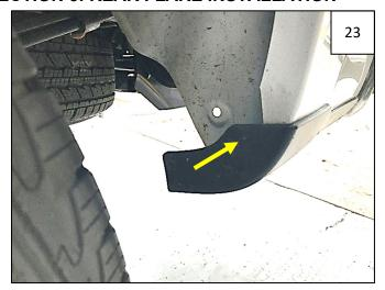
Remove 1 factory T15 Torx screw on rear splash guard. Retain all factory screws; some will be used.
