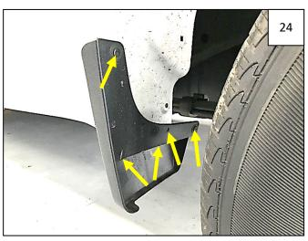
Remove 5 factory screws from the front splash guard. Splash guard is held on with a hidden clip – to remove, pull splash guard firmly from vehicle.
