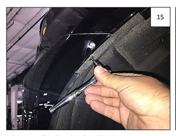
Remove 1 T15 Torx bolt from front bumper as shown. Retain bolt for use in next step.
