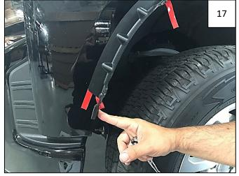
Lower tab of Inner Bracket must be flush against fender well as shown before pulling tape leaders.
