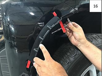
Make sure tape leaders on Inner Bracket are folded outward in both directions. Hold Front Inner Bracket on Bumper and reinstall T15 Torx screw removed in Step 15.
