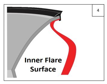
Peel 2-3 inches of red vinyl backing away from supplied edge trim tape. Applying the adhesive side of the edge trim to the inner side of the flare, affix the edge trim to the top edge of the flare (the portion that comes in contact with the side of the vehicle).
