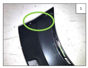
Extension pieces look very similar so make sure to check markings on each part and use those made for your vehicle model. Marking on part is located in circled area.
