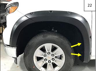
Start 2 factory T15 Torx screws at bottom rear of wheel well as shown. Apply pressure to flare towards vehicle body at each fastening point and tighten all fasteners.
