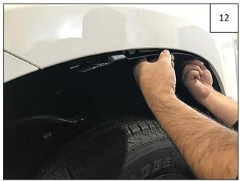
Install Top Inner Bracket using 2 T15 Torx screws retained in Step 11. Tighten both fasteners. **NOTE:** Driver Side bracket is marked with LH, Passenger Side is RH.
