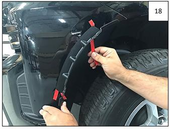
Holding lower tab in place, pull leader from lower tape on Inner Bracket. Press part to adhere.
