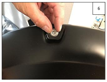
Insert Push-In Pocket Hardware into each flare pocket hole (on outer flare surface, 8 places each front flare, 9 places each rear). Push in to engage clip and tape adhesion.
