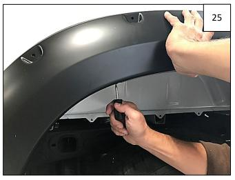
Align the flare on the fender and mark 3 holes using a grease pencil.
