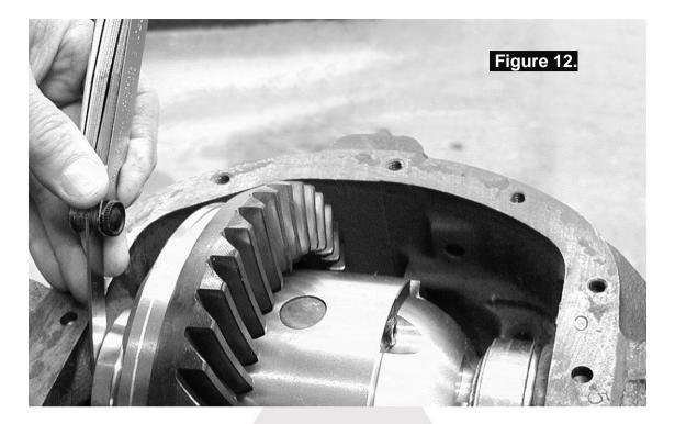
Add the specified preload amount to the end float measurement determined with the feeler gauge to determine a shim amount for 'E' (Refer to Figure 11.).
