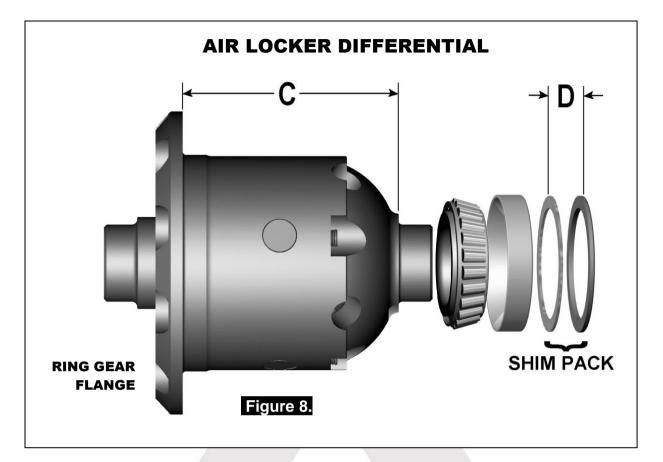
☐ Measure the distance from the *Air Locker* bearing shoulder to the ring gear mounting face (shown as '**C**' in Figure 8.) and record this measurement as '**C**'.
