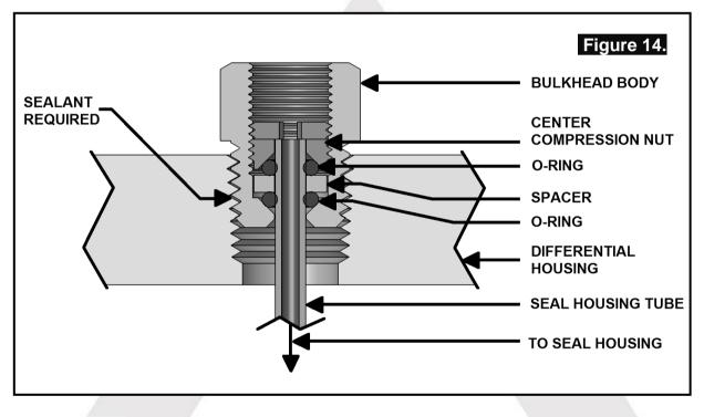
NOTE : Make sure the seal housing tube is all of the way into the center compression nut while you are tightening it.
