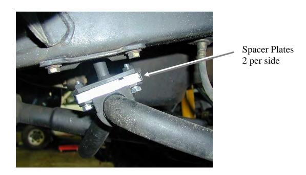
This kit is used to space the front sway bar away from the tail shaft when the suspension is in full droop.
