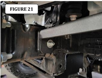
**Step-31** Adjust your bumper to square up with the front end and fasten any loose hardware accordingly. The wings of the bumper should line up where the fender and OEM bumper meet.
