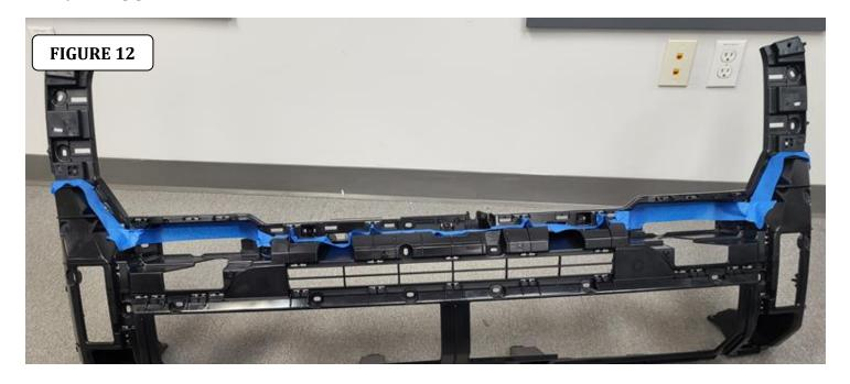
**Step-17** Proceed to cut out the plastic frame and the end caps previously removed.
