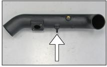
16. Install the provided 3/8" hose fitting into the K&N® intake tube as shown.
