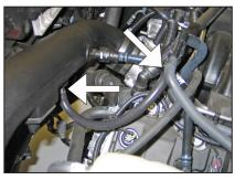
24. Install the provided silicone hose onto the 3/8" fitting installed in the K&N® intake tube and then attach the open end to the EVAP check valve.
