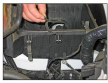
12. Remove the center airbox retaining clip.
