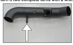
17. Install the provided quick disconnect fitting into the  $K\&N^{\otimes}$  intake tube as shown.
