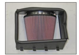
11. Install the K&N® air filter onto the filter adapter and secure with the provided hose clamp.
