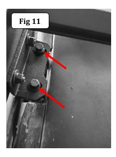
**Step-11** Adjust and align the Ceros roof rack assembly as necessary and fully tighten all hardware.
