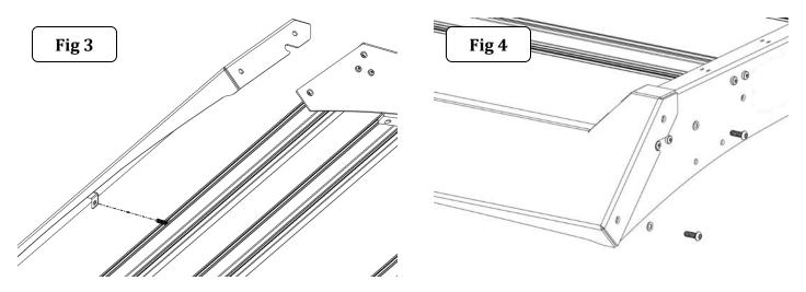
**Step-5** Begin the brackets assembly on the passenger side, install (2)  $\frac{1}{4}$ " x 1" SEMS button screws in the front holes of the side rail. Place the front bracket onto the side rail, align the screws with the holes in the front bracket. Secure the front bracket using (2)  $\frac{1}{4}$ " flat washers and (2)  $\frac{1}{4}$ " hex nuts. Snug but do not tighten the screws, (Fig 5).
