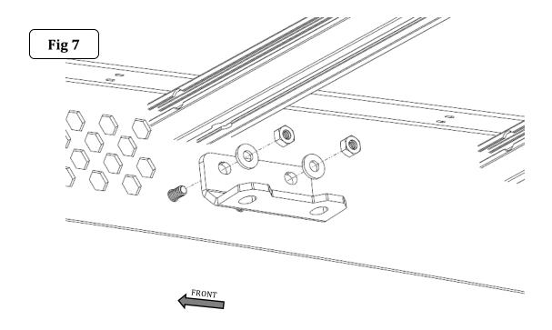
**Step-7** Repeat Step 5 and 6 to attach the brackets to the side rail on driver side.
