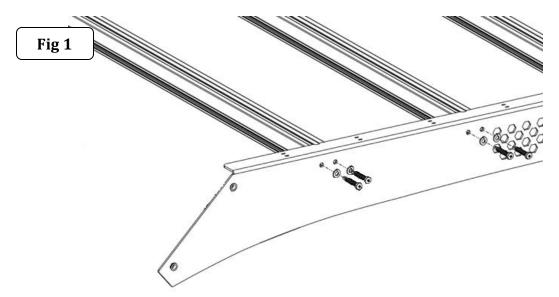
**Step-3** Install (3)  $\frac{1}{4}$ " x  $\frac{3}{4}$ " hex bolt in the channel of the front crossbar that will be facing forward when the Ceros roof rack is fully assembled. Position one bolt at middle of the crossbar and other on each side (Fig 2).
