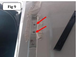
Step-9 Place the spacers on the roof rail over the factory nuts (Fig 10).
