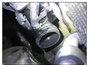
5. Install the provided hose clamps onto one of the provided step coupler as shown and then install the coupler onto the turbo inlet and secure with the hose clamp.
