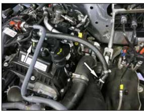
20. Install the CCV hose assembly onto the valve cover and turbo inlet tube fittings.
