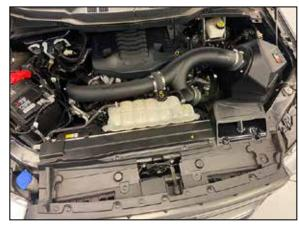
22. Reinstall the air filter housing and intake tube. NOTE: Shown with K&N intake kit 63-2617 installed.
