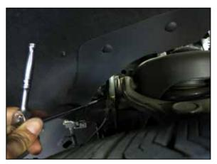
3. Remove the passenger side turbo inlet tube by accessing the hose clamp on the turbo inlet through the passenger side wheel well. Lift the splash shield up and use a ratchet, extension with 7mm socket.
