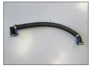
19. Assemble the provided CCV hose as shown.
