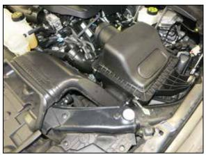
2. Loosen the three hose clamps that secure the intake tube to the air filter and turbo inlet tubes and then remove the tube from the vehicle. Remove the bolt that secures the air filter housing to the inner fender, lift the air filter housing up to dislodge it from the mounting grommets and remove it from the vehicle.
