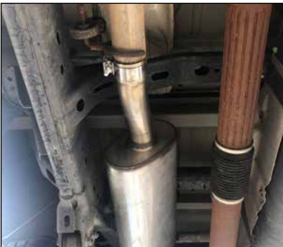
8. Slide the inlet clamp on to K&N muffler assembly. Then slide muffler assembly onto midpipe followed by inserting muffler hangers into insulators. NOTE: Do not tighten the muffler inlet clamp at this time. Install clip with stainless steel braid on muffler hanger and then slide clamps on to muffler outlets.
