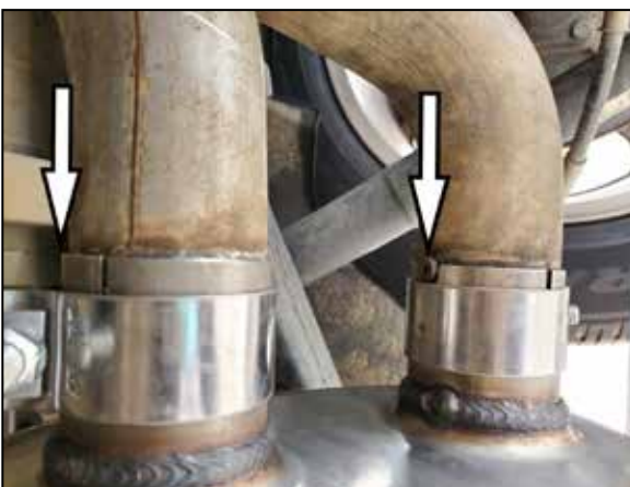
9. Insert driver/passenger side tailpipe into muffler outlet, then slide rubber insulators onto tailpipe assembly and then to the frame hangers. Do not tighten clamp at this time. Ensure that each tailpipe assembly is fully inserted with locating pins aligned.
