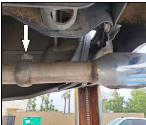
11. Double check to make sure everything is tight and properly positioned before lowering vehicle to the ground. NOTE: If necessary, the TIP assemblies can be adjusted via conical clamp near the end.
