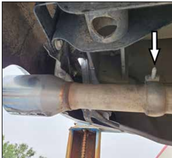
10. Check alignment of driver and passenger tip assembly and reposition as necessary. Once final position is satisfactory, tighten all hardware and band clamps from front to rear of vehicle. Ensure that the band of the clamp is covering the "Z-notch" of each inlet and outlet to avoid leaks. Clean exhaust tip of any finger prints or grease marks. NOTE: All band clamps should be torqued to 40-45 ft-lbs.
