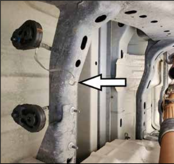
7. Remove the small clip attached to the stainless-steel braid in front of the rubber. Now remove the muffler from the rubber insulators (leave insulators on frame side).
