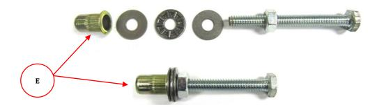
**Step-5** Place the nut-sert with the attached tool components into the enlarged hole. Use a 7/16" wrench to hold the nut, and tighten the bolt using a 7/16" wrench or socket and ratchet. Continue tightening the bolt until the Nut-Sert is fully compressed and no longer spins. Remove the tool components and Install a nut-sert into each of the remaining holes that were enlarged.
