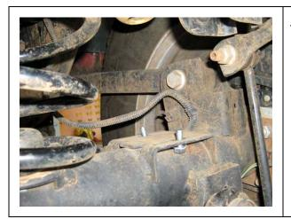
1. Fit 2 M8 x 20 bolts with flat washers to bump stop plate from underside as shown.
