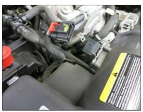
3. Disconnect the mass air sensor electrical connection and set aside, lift the air filter housing up to dislodge it from the mounting grommets and remove it from the vehicle.
