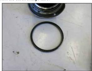
14. Remove the sealing O-ring from the factory charge tube.
