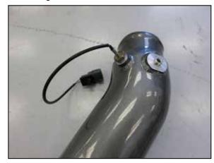
17. Remove the temperature sensor from the factory charge tube and install it into the K&N upper charge tube. Install the provided 1/8npt plug into the accessory port. **NOTE: Apply thread sealer to the 1/8npt plug before installation.**
