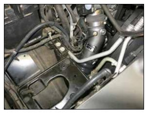
23. Reinstall the factory air filter housing support bracket and mounting plate using the factory bolts.
