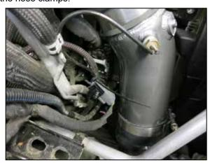
21. Reconnect the charge tube temperature sensor electrical connection.
