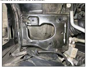
4. Remove the four bolts that secures the air filter housing mounting plate and then remove the plate from the vehicle.
