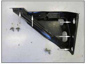
5. Remove the five bolts that secure the support bracket for the air filter housing mounting plate and remove the support bracket.
