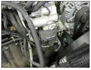
18. Install the provided single hump coupler onto the throttle body and secure with the provided hose clamp.
