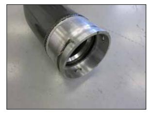
16. Install the factory locking ring into the K&N lower charge tube.
