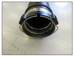
11. This picture shows the security and locking clip in the unlocked position after the charge pipe is removed.
