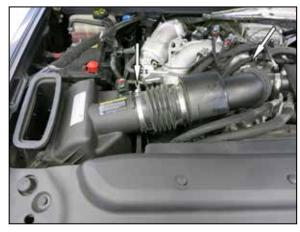
2. Loosen the two hose clamps that secure the factory intake tube to the turbo inlet and air filter housing, then remove the intake tube from the vehicle.
