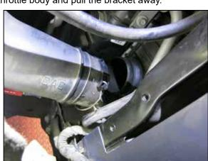
10. Using two flat blade screw drivers, pry out the black security clip and pull back to separate the charge tube from the intercooler. Remove the charge tube from the vehicle.
