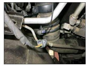
6. Disconnect the charge tube temperature sensor electrical connection.
