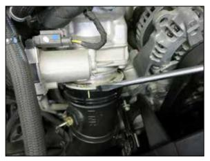
8. Using a flat blade screwdriver or similar device, rotate the locking ring that secures the charge tube to the throttle body while applying pressure down on the charge tube until the tube separates from the throttle body.
