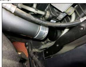
19. Install the lower K&N charge tube onto the inter cooler, Push the tube until an audible "click" is heard ensuring the locking ring has locked into position. Verify the tube is locked on by pull back to see if the ring is engaged.
