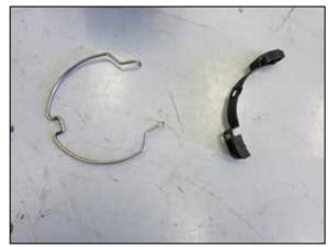
13. Remove the black security clip and locking clip from the stock charge tube.
