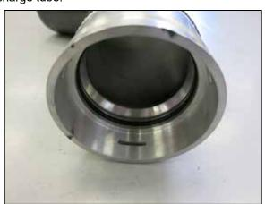
15. Install the factory sealing O-ring into the K&N lower charge tube.
