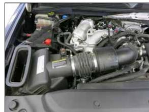
24. Reinstall the intake system and reconnect the mass air sensor electrical connection.
