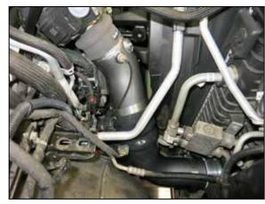
20. Install the K&N upper charge tube, double hump coupler and clamps onto the K&N lower charge tube and the coupler at the throttle body. Adjust all parts for best position and then tighten the hose clamps.
