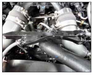
21. Unsnap and remove the plastic cover over the wiring harness.
