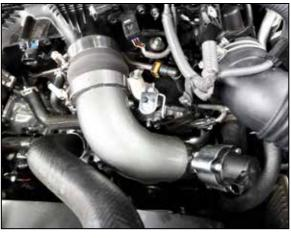
15. Install the driver side K&N charge tube into the factory lower coupler, align with the upper hump coupler and install. Secure with the factory lower clamp and the upper hose clamp provided.
