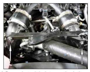
3. Remove the two bolts that secure the plastic wire harness cover and then disconnect the five sensors that the harness connects too.
