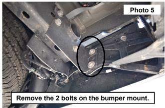
Photo 6 Photo 5 Remove the 2 bolts facing the bumper.
