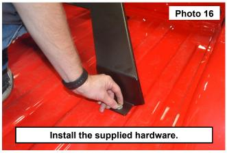
3/8 lock washers and (4) 3/8-16 nuts. Torque to 35 ft-lbs. using a 9/16 wrench and socket. **See Photo 17.** 18. Install the wheel and tire onto the carrier secure using the supplied lug nuts. **See Photo 18.**
