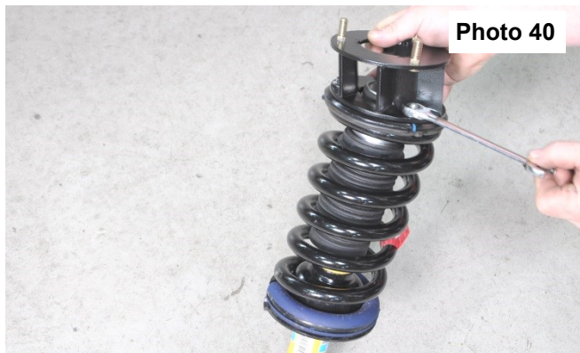
Install Strut Spacer on Strut with Shorter Side to Inside
