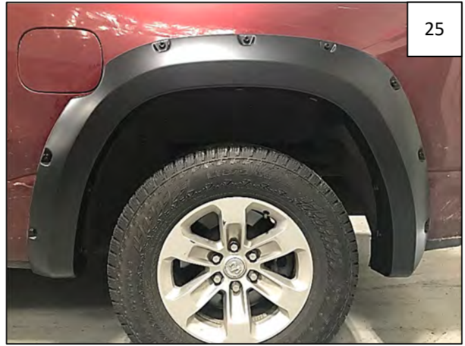
Complete Rear Flare Installation.
