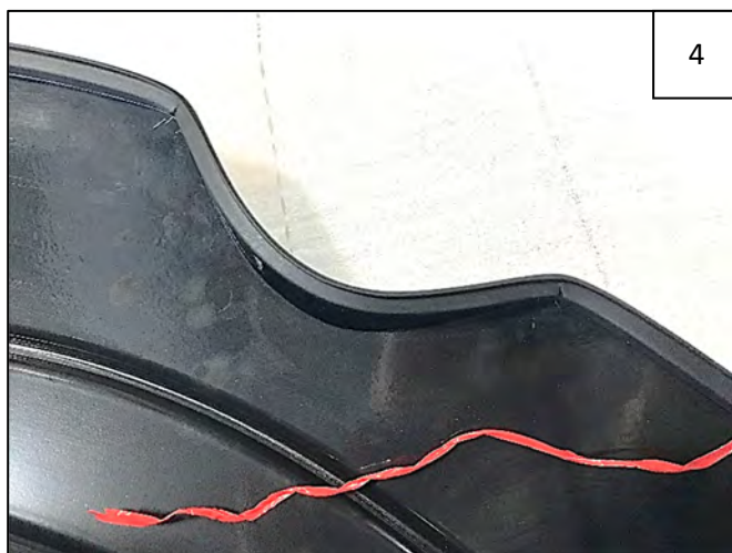
Correctly-installed edge trim around gas door.
