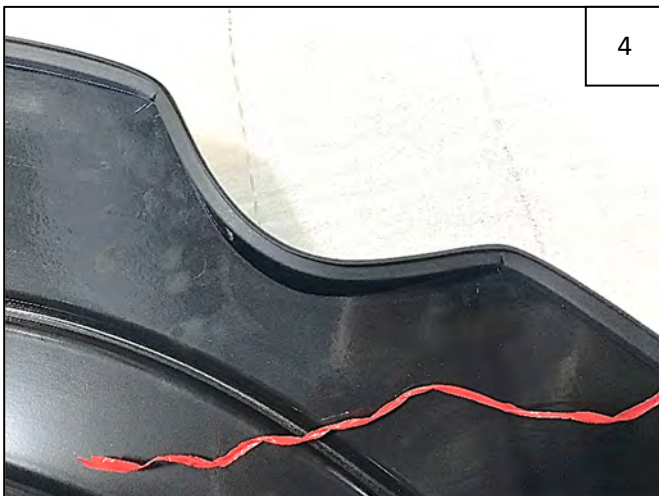
Correctly-installed edge trim around gas door.
