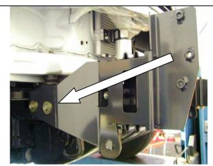
7. Mount the Impact Absorber brackets to each side of the chassis using original fasteners.
