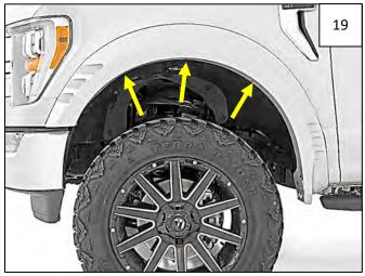
Aligning flare on fender, press inward, firmly with force, on the flare to line up the flare mounting holes with the clips on the Inner Bracket. Install 3 supplied #10 Truss-Head Screws through the flare and into the Inner Bracket. Do not tighten.
