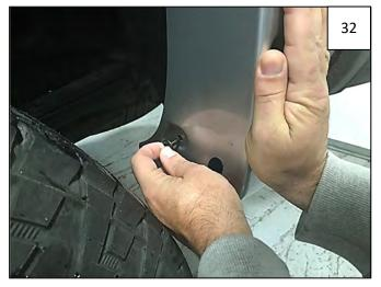
If you removed both factory plastic fasteners in Step 25, install 2 supplied Plastic Retainers through flare and into factory holes at rear of wheel well.
