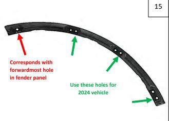
Line up Inner Bracket holes shown in Step 18 starting with the forwardmost hole in the fender panel and continuing with clips installed in Step 13. Inner Bracket will follow the curvature of the wheel well.
