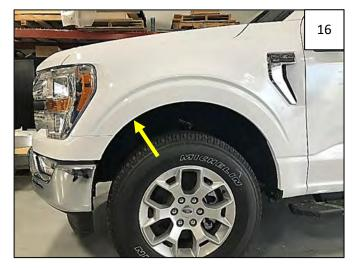
Using a 7mm socket, reinstall 1 factory screw through the Inner Bracket and into fender.
