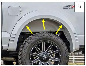
Install 3 supplied #10 Truss-Head Screws through upper holes in flare and into clips installed in Step 29. Apply pressure to flare towards vehicle body at each fastening point and tighten all fasteners.
