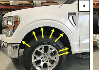
**If your vehicle is 2021-2023**, use 7mm socket to remove 7 factory screws from wheel well. Retain all screws for reinstallation.
