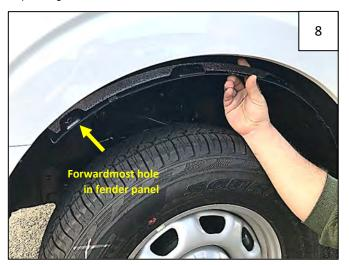
**For 2021-23 vehicle**: Line up Inner Bracket holes show in Step 12 with 4 holes in wheel well, starting with the forwardmost hole in the fender panel (not the bumper). Inner Bracket will follow the curvature of the wheel well.
