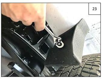
Remove a  $3^{\mbox{\tiny rd}}$  screw from underside of lower front of wheel well.
