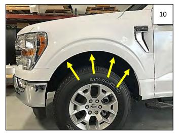
Using a 7mm socket, reinstall 4 factory screws (and/or additional supplied #8 Truss-Head Screws) through the Inner Bracket and into fender. Tighten these screws.
