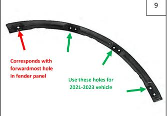
Holes to be used to install Inner Bracket for **2021-2023 vehicle** (forwardmost of each pair of holes).
