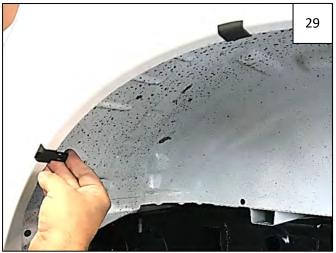
Slide a supplied Long "U" Clip over each foam tab. Clip will overhang wheel well lip on both inner and outer surface. Clip hole should be centered approximately over mark made in Step 26.
