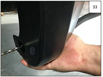
If your model does not have an outer plastic fastener, hold the end of the flare firmly on fender and drill a 1/4" hole through lowermost hole, into plastic trim. Hole should align with hole in sheet metal. Install supplied Plastic Retainer.
