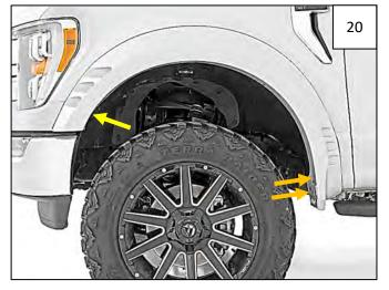
Still pressing flare firmly to fender, reinstall 4 remaining factory screws removed in Step 4 or 5 (depending on model year). Apply pressure to flare towards vehicle body at each fastening point and tighten all fasteners.
