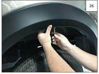
Holding flare firmly on fender, aligning holes in flare with fender lip. Mark 3 hole locations on fender lip with a grease pencil.
