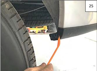
Using a pry tool, remove both factory plastic fasteners from lower rear of wheel well. Discard.
