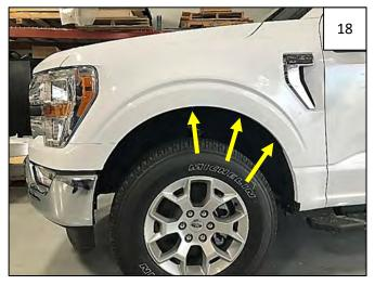
Using a Phillips Screwdriver, install 3 supplied #10 Truss Head Screws through 3 remaining holes in Inner Piece and into clips installed in Step 13. Tighten all screws.
