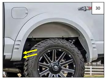
While holding flare to vehicle, start 2 factory screws in lower front of wheel well.
