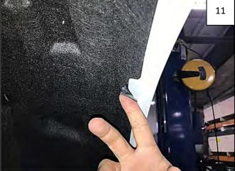
**For 2024 vehicle**: Peel backing from supplied Foam Tab. Wrap a Foam Tab over each interior fender tab, locations shown in next step (certain vehicles may or may not have factory holes in fender tabs; these will not be used).
