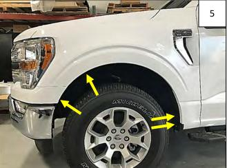
**If your vehicle is 2024**, use 7mm socket to remove 4 factory screws from wheel well. Retain all screws for reinstallation.
