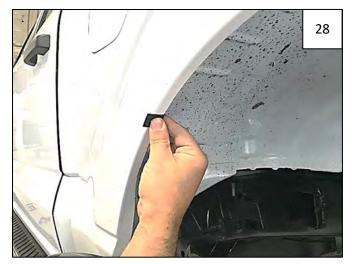
Peel backing from supplied Foam Tab. Center a Foam Tab over each mark made in Step 26, folding each tab over the wheel well lip. Press to adhere.
