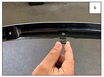
Install 3 Plastic Panel Clips onto the Inner Bracket as shown. **NOTE:** Driver's side Inner Bracket is marked with an "LF" and the passenger's side Inner Bracket is marked with an "RF".
