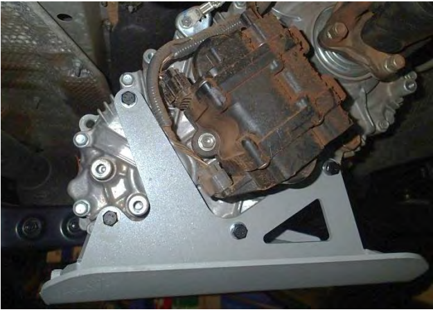
Transfer case panel rear side
