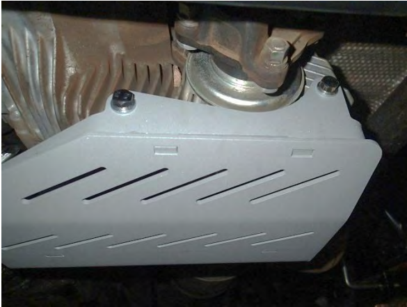
Transfer case panel front side
