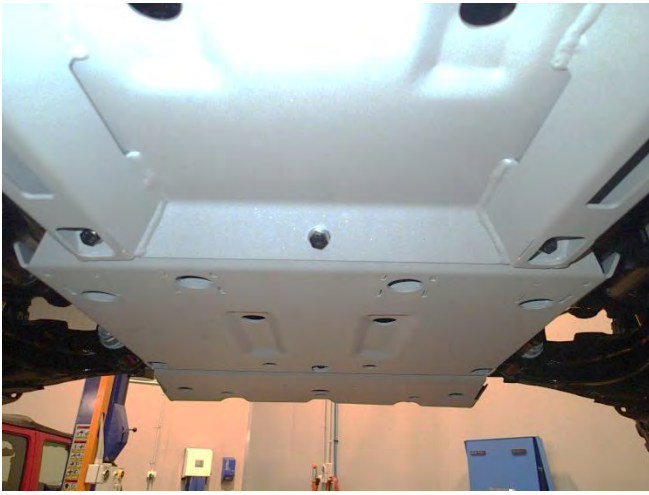
Connect transmission panel
