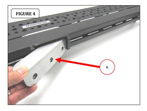
**Step-4** Attach the driver side Dominator running board to each bracket using (2) 3/8" x 1  $\frac{1}{4}$ " hex bolts, (2) 3/8" lock washers, (2) 3/8" flat washers, and (1) 3/8" Nut-Plate (FIGURE 5).
