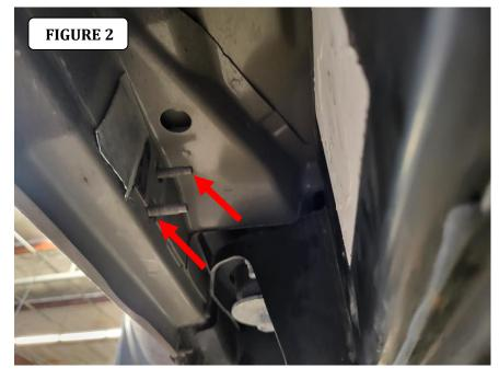
**Step-2** Attach the driver side brackets to the underside of the body using (2) M8 lock washer and (2) M8 flat washer, and (2) M8 hex nut, on each bracket (FIGURE 3). Leave the nuts loose for final adjustment.
