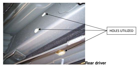
Place an 8mm x 20mm Hex Head bolt (C) through running board bracket (B) and start the bolt into a M8 – 1.25 2 tab weld nut (F) in the front hole location shown below. Then start the 2 rear hole location bolts (shown below) into a M8 – 1.25 single tab spot weld nut (G). Position bracket into front driver location with thread plates in vehicle openings and tighten, but do not tighten completely.
