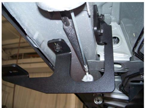
Place running board (A) onto the brackets. Align 8mm square head bolts (E) in the bottom of the running board (A) with holes in the brackets. Completely tighten brackets to vehicle. Center board on vehicle between wheel well openings or until desired appearance is aquired. Adjust board in/out on vehicle until desired appearance is met. Secure board into palce using 8mm hex nuts (D).
