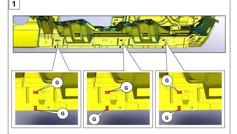
NOTE: FOR STANDARD CAB APPLICATIONS, MIDDLE BRACKET LOCATION IS NOT AVAILABLE. PROCEED AS DIRECTED USING FRONT AND REAR MOUNTING LOCATIONS. EXTRA BRACKETS AND HARDWARE MAY BE DISCARDED.
