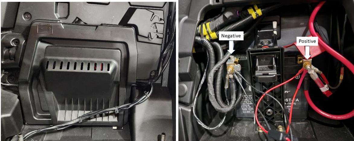
Remove the battery cover by pulling outward from the top. Using a 10mm wrench, remove the negative battery cable followed by the positive.
