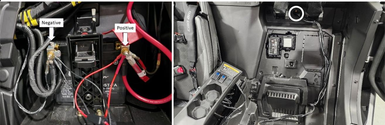
Reattach the positive cable of battery and the positive ring terminal of the harness. Repeat with the negative cables. Use zip ties to place one of the light leads into a small service loop. Run the second lead out of the battery compartment, up the firewall and through the pass through (circled). Plug the connector into the light and secure the wiring with zip ties. Bundle excess wires and secure in the battery tray.
