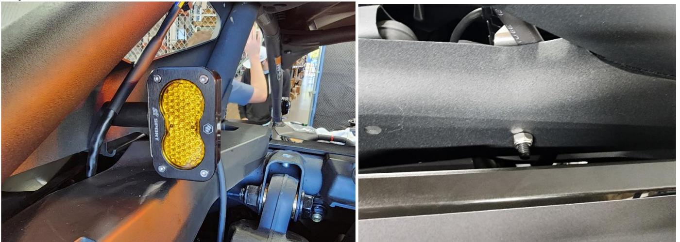
Place the 1.75" spacer on the M6 bolt and slide the bolt through the B-Pillar. Secure it with the ¼" washer and M6 nylock nut. Tighten using the 10mm wrench and socket.
