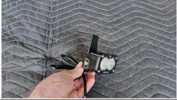
**Step 2:** Place a M6 Hex Screw (20-1243) and a M6 Washer (20-1141) inside both lift point frame hole going through the <u>inside hole</u> with the threads facing down. Align the Reverse Bracket (Left = 44-7684 and Right = 44-7685) bottom mounting holes (near the letter identifier) with the screw and secure it to the frame with a M6 Washer (20-1141) and M6 Locknut (20-1690). Loosely tighten the nut so that the top mounting point can be adjusted if necessary.
