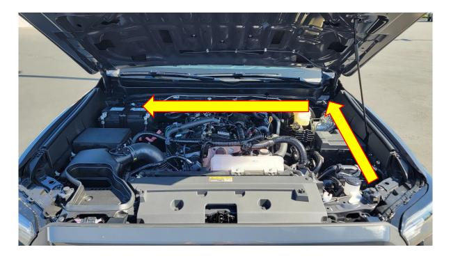
**Step 11 Toggle Only:** Using a 10mm and 12mm socket, disconnect both the negative and positive battery cable. Locate the red ring terminal of the Off/On harness (64-0139) and attach it to the positive battery post using a 12mm socket. **(for hybrids, refer to hybrid instructions)** Secure the relay near the battery.
