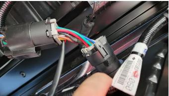
**Step 7 Toggle Only:** Remove the protective cap from the connector at the rear frame powered circuits junction box of the vehicle (A) -> (B). The junction box is located underneath the vehicle near the rear left (drivers' side) taillight. Connect the Rear Circuit Output Adapter (60-0103) to the Splitter harness installed in step 6 and to the OEM Junction Box (C). Tie all loose wiring neatly away from hot, rotating or sharp components using the provided Zip-Ties (20-1612).
