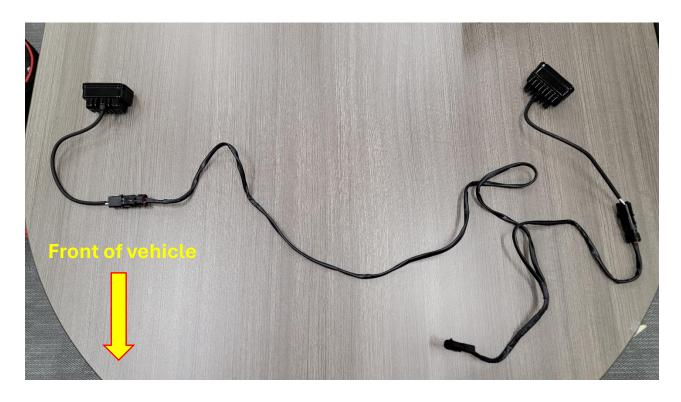
**Step 7 (For Plug and Play Only):** Connect the 2-Pin Hitch Mount Light Adapter Harness (60-0068) by removing the OEM hitch plug and inserting the harness in between. Once connected, connect the Splitter Harness installed in step 6. Tie all loose wiring neatly away from hot, rotating or sharp components using the provided Zip-Ties (20-1612). Test installation by turning on vehicle and putting it in reverse. Installation is complete!
