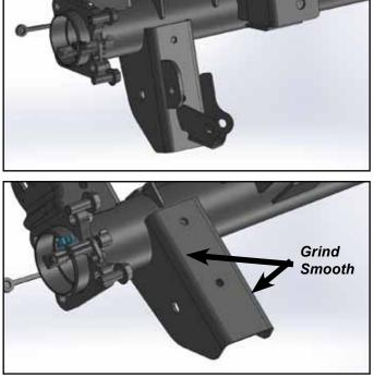
• Measure down from the factory lower control arm hole 1-3/8" and mark a horizontal line. Trim and remove this section from the vehicle.
