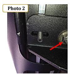
**Step-3** Align the side step with the vehicle and tighten all brackets and side steps nuts and bolts. Repeat the above steps to install the passenger side brackets and side step. Remember to check and retighten the nuts and bolts every six months.
