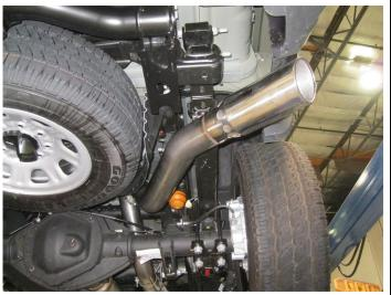
**Step 3.** Next Install the Tail Pipe Assembly in a similar fashion using the supplied 4.00" clamps and by fitting the welded hangers into the rubber insulators.
