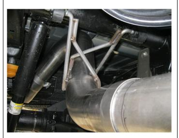
**Step 2.** Begin installation of the Magnaflow system by clamping the Inlet Pipe to the newly cut outlet of the DPF using a supplied 4.00" clamp and fitting the hangers in the rubber insulators (leave all clamps loose for final adjustment of the complete system). If your vehicle has an O2 sensor re-install at this time. If not, install the provided sensor boss plug.
