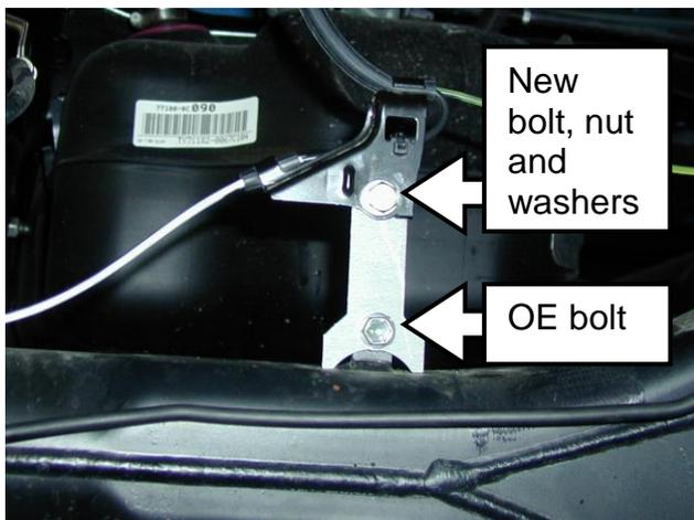
2. Fit relocation plate to axle housing using OE bolt as shown.
