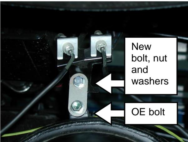
2. Fit relocation plate to axle housing using OE bolt as shown by arrow.
