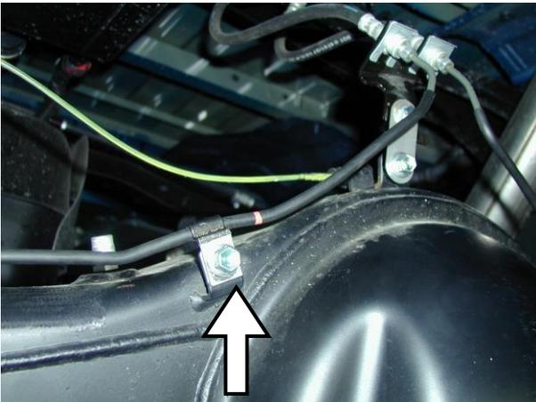
4. Rotate clip shown by arrow so that the brake line is positioned above the bolt.
