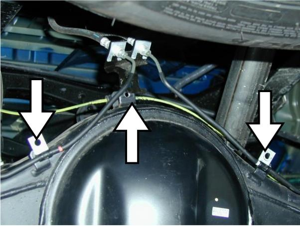
1. Remove bolts securing brake line as shown by arrows.
