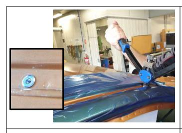
Using a nutsert gun, fit nutserts to the front and rear holes on both roof gutters as shown.
