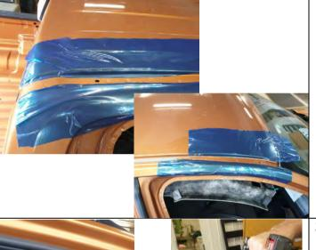
19. Use low tack film or similar to protect the areas around holes that need drilling as shown.
