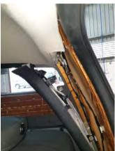
3. Pull back the door seal on the top half of the door jamb. Unclip and pull back the side rear pillar trims on both sides as shown.
