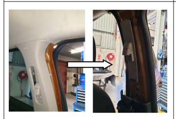
6. Unclip and remove the B-pillar plastic trim on both sides.
