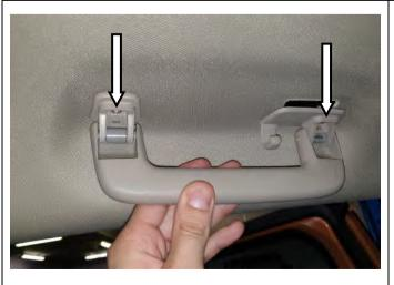
4. Remove the rear grab handles. This is done by removing plastic covers to expose the torx head screws.
