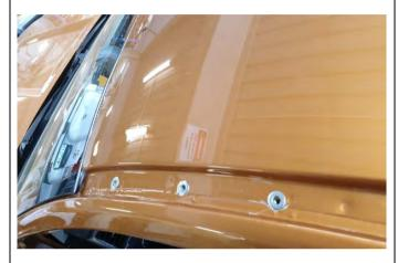
Note: Ensure the nutserts are done up tight. If they are not installed correctly, they may leak.
