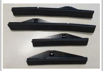
29. Fit the foam seal on the feet. Using a 7.0mm drill bit, drill through the mount feet holes to open up the foam seal.
