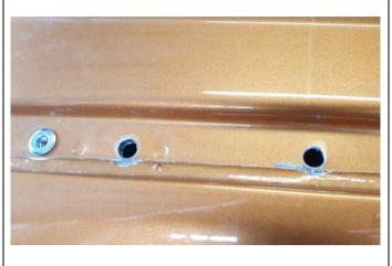
26. Remove any roof seam sealant that is going to interfere with the heads of the nutserts using a small flat blade screwdriver as shown. Use anticorrosive touch up paint on any exposed areas.
