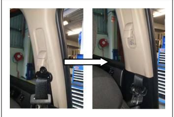
5. Remove the plastic cap to expose the retaining bolt on both front seat belts as shown.
