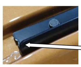
Temporarily bolt the front mount feet in place using M6x25 bolts and washers in the front hole. It is critical that the identification notch faces the front of the vehicle.
