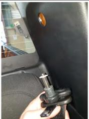
2. Undo the torx head bolt on each side rear seat belts and remove. Allow the seatbelt to hang down as shown.
