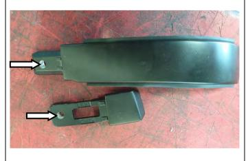
18. Drill out the threaded holes on the end trims to 7.0mm as shown.
