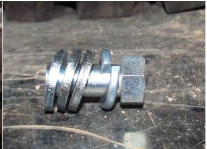
Figure 2: washers on female bolt
